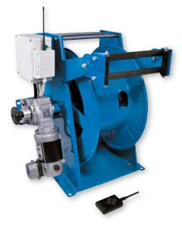
Hose reel, available in painted or in stainless steel AISI 304, with **electric 12 VDC - motor for hose rewind.** The motor is connected to an external reduction gear with clutch torque limiter. Suitable for hoses of max 100 m length in 1/2".
