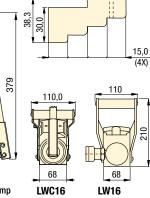
▼ For lifting heavy equipment with minimum floor clearance the LW16 is the ideal tool.
