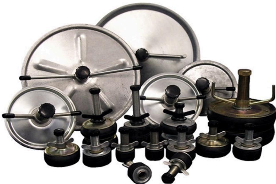
These are provided in sizes from 1.5", for more strenuous effort oriented duties such as long immersion in water and higher temperature. The plugs are merely inserted into the pipe and the wings tightened to force the top and bottom plates together, thereby expanding the rubber ring to seal tightly in the pipe.
