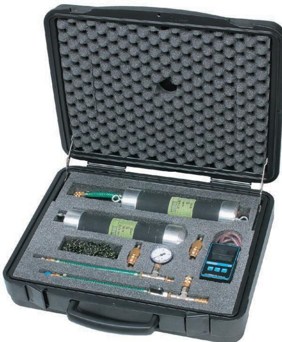
This set is used for DN 80 to 150 mm pipe leak tests using air as the testing medium. They can be used both in straight sections of the pipe and in section with round or sharp bends or knee pieces up to 90 degrees. The set consists of a digital pressure gauge and all the necessary fittings and accessories for carrying out leak tests according to DIN EN 1610.
