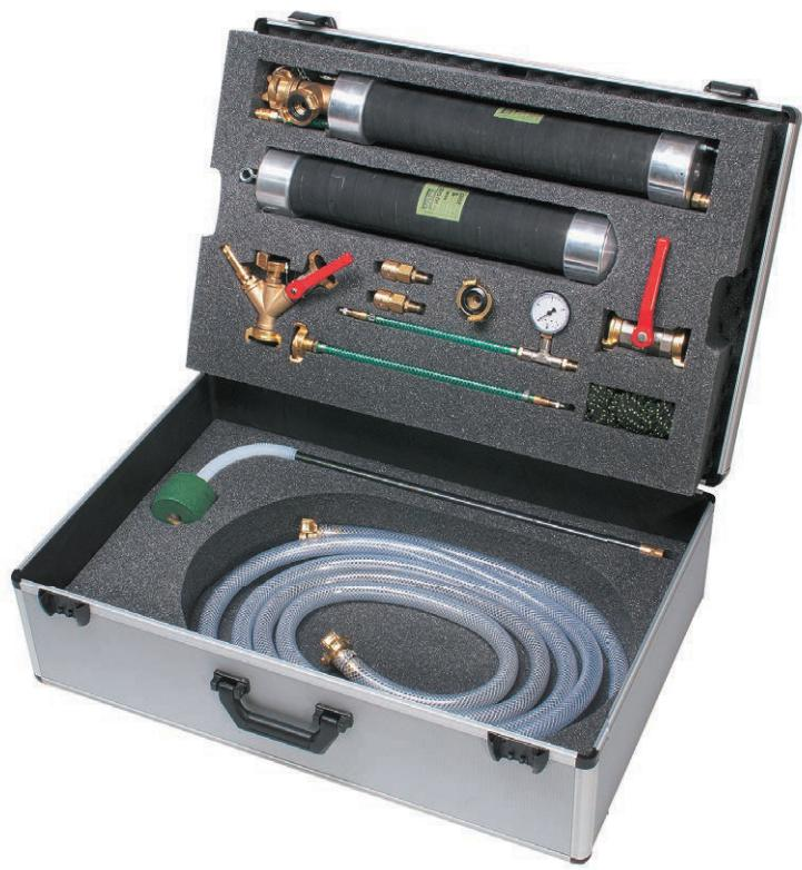
This set is used for DN 100 to 200 mm pipe leak tests using air or water as the testing medium. They can be used both in straight sections of the pipe and in section with round or sharp bends. The set consists of all the necessary fittings and accessories for carrying out leak tests according to DIN EN 1610.
