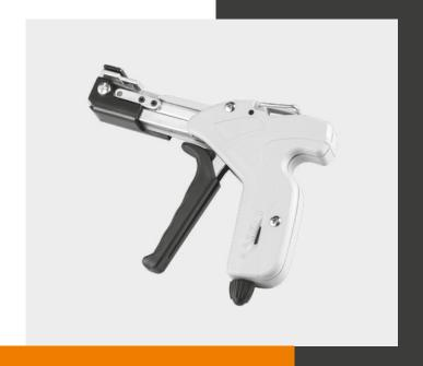
The tool is used to quickly and economically install stainless steel ball-lock cable ties. It automatically cuts ties up to 7.9 mm wide and 0.3 mm thick. It also enables adjusting the tension with a knob located on the bottom of the handle.
