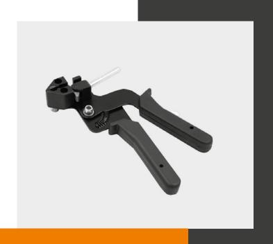
Tool for tensioning and cutting stainless steel cable ties. Resistant to corrosion and oxidation. Ideally suited for Ball-lock ties made from various grades of stainless steel. The handle can be used to adjust the level of tension on the tie as needed, the built-in mechanism cuts off the excess section of the tie.
