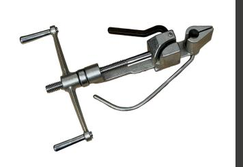
The XL screw strapping device is a special tool used for tensioning stainless steel straps with a thickness of 1 and 1.2 mm and a width of 19, 25 and 32 mm.
