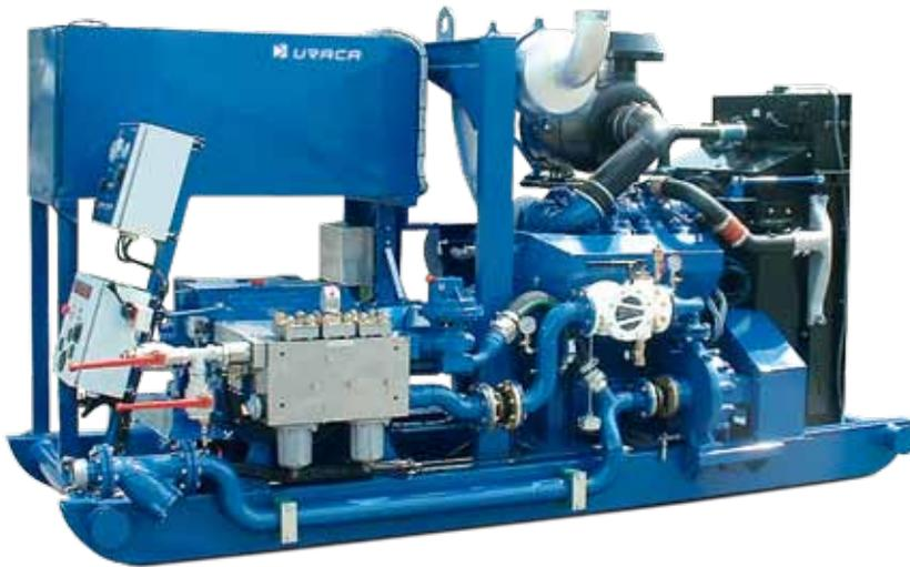
Diesel driven test pump unit DP725 D.
